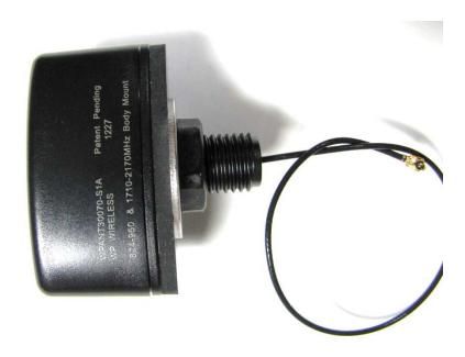
Note: The screw mount has two flat edges on opposite sides.
